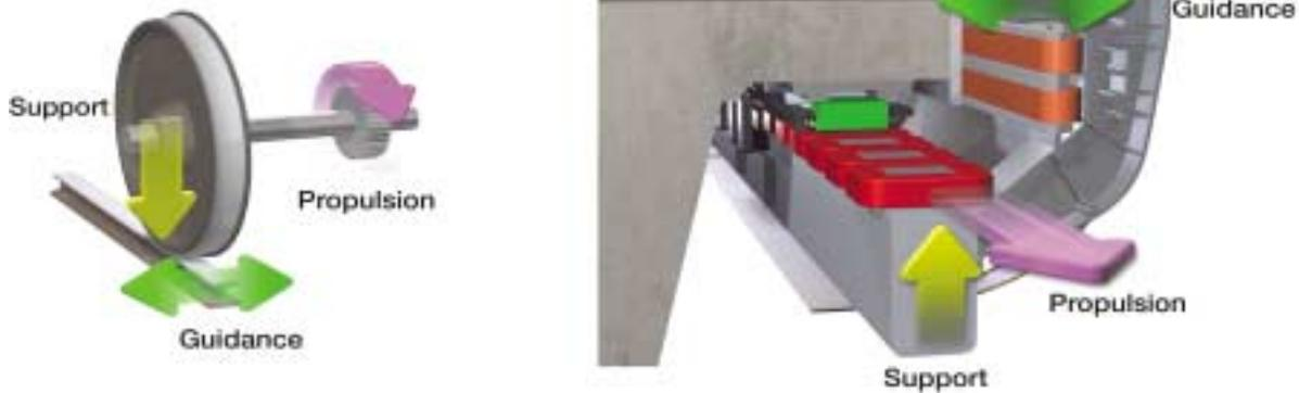
**A comparison of the fundamental properties of a traditional rail system (left) and a maglev system (right).**
